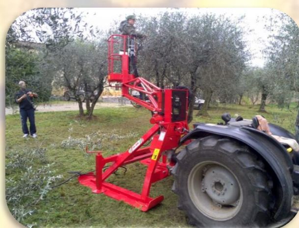
TR1K used for the pruning of low olive trees
