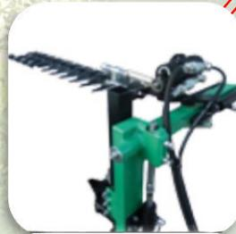
Topping horizontal superior bar with inclination
