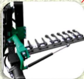
Horizontal lower with hydraulic inclination
