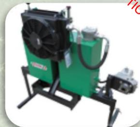
Hydraulic system to be applied to an all-purpose tractor
