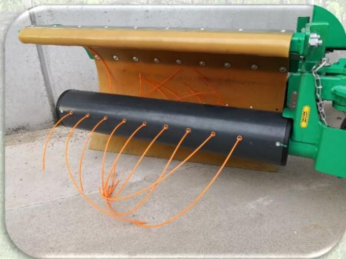
Roller with 9 reels of 9 MT of wire Ø 4 mm
