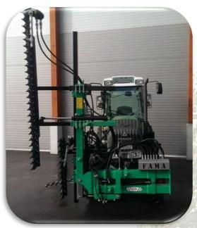
CKP2BV. Looping machine with 2 vertical cutting planes (2 + 1 Mt.)
