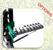
Horizontal lower with hydraulic inclination
