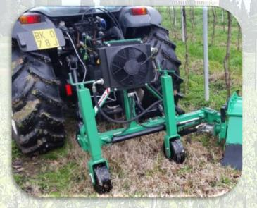
**ECO TRIMMER "SPECIAL" Model:** Version with out pipes that make the roll's translation. Frame with 3 points connection with hydraulic cylinder for the header stroke translation, 2 stabilizing wheels adjustable in height, heater exchanger.
