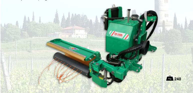
"ECO TRIMMER 1" Model: Frame with 3 points connection with hydraulic cylinder for the header stroke translation 50 cm, 3 stabilizing wheels adjustable in height, heater exchanger, header inclination control for leveled operation based on the slope of the ground.
